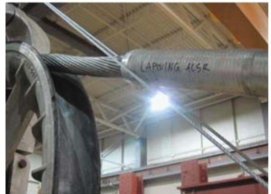
Different conductor sizes were incorporated into the test program. Each connector ran through the traveler numerous times before final testing.
