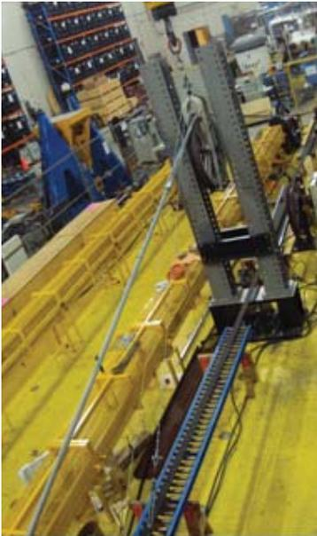
The test program was designed to simulate a splice passing through a traveler. In the test setup, a traveler was suspended from an overhead crane to replicate a field application. Numerous harsh conditions were then tested, pushing the connections to the extreme.
