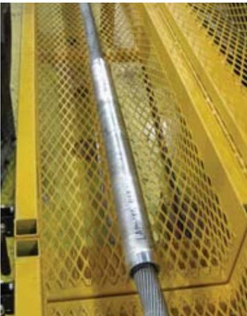
Pull testing of the complete assembly allowed for final performance evaluation. If the conductor were to maintain close to or better than its original rated strength, then the extreme application would prove IMPLO to be capable of passing through the traveler in application.
