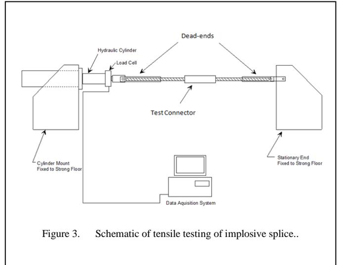
Figure 3. Schematic of tensile testing of implosive splice..
