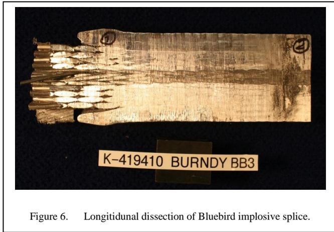
Figure 6. Longitudinal dissection of Bluebird implosive splice.
