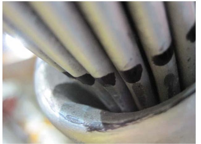
Figure 4. Localized conductor strand flattening at 50 degree tensile test. (1590 ACSR Lapwing splice)
