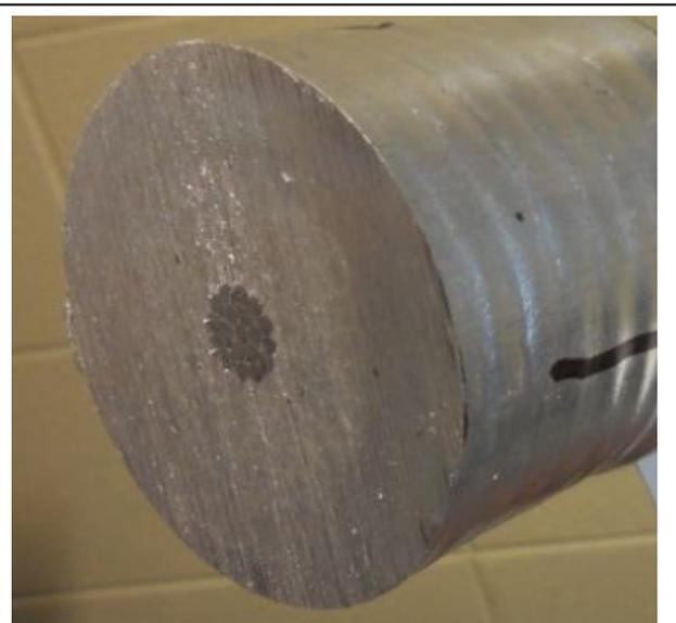
Figure 5. Cross-sectional dissection of Bluebird implosive splice.
