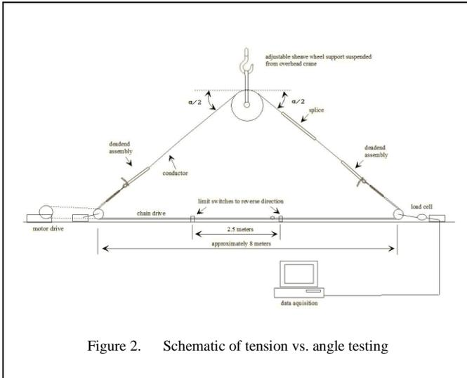
Figure 2. Schematic of tension vs. angle testing
